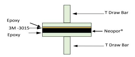
Figure 1. Sample set-up for Adhesion Testing
